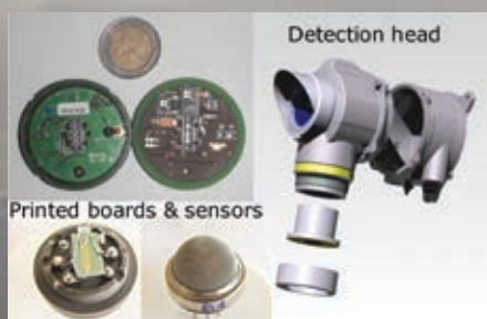
Top left: Photos of electronic boards. Bottom left: a sensor with and without a head grid. Right: Simtronics' detection head.
